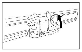
The adapters are used to hold the net. Slide the adapters to the desired location on the upper and lower groove of the rail and turn the handle up to lock it in place. Compress the rods of the net and insert them into the corresponding openings of the adapter. The longer rod is for the upper adapter.
